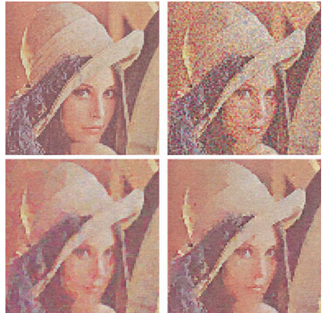
Figure 7. Left to right, top to bottom: original, noisy, TV and Beltrami images.
